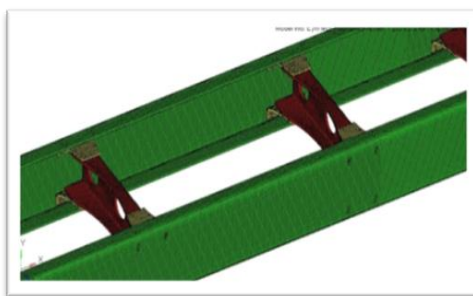
Fig.3 Meshed chassis frame
